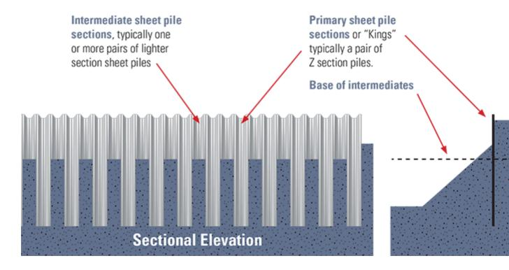
KSP walls are normally designed for use with Z piles. U piles do not work efficiently in a non-continuous wall.
